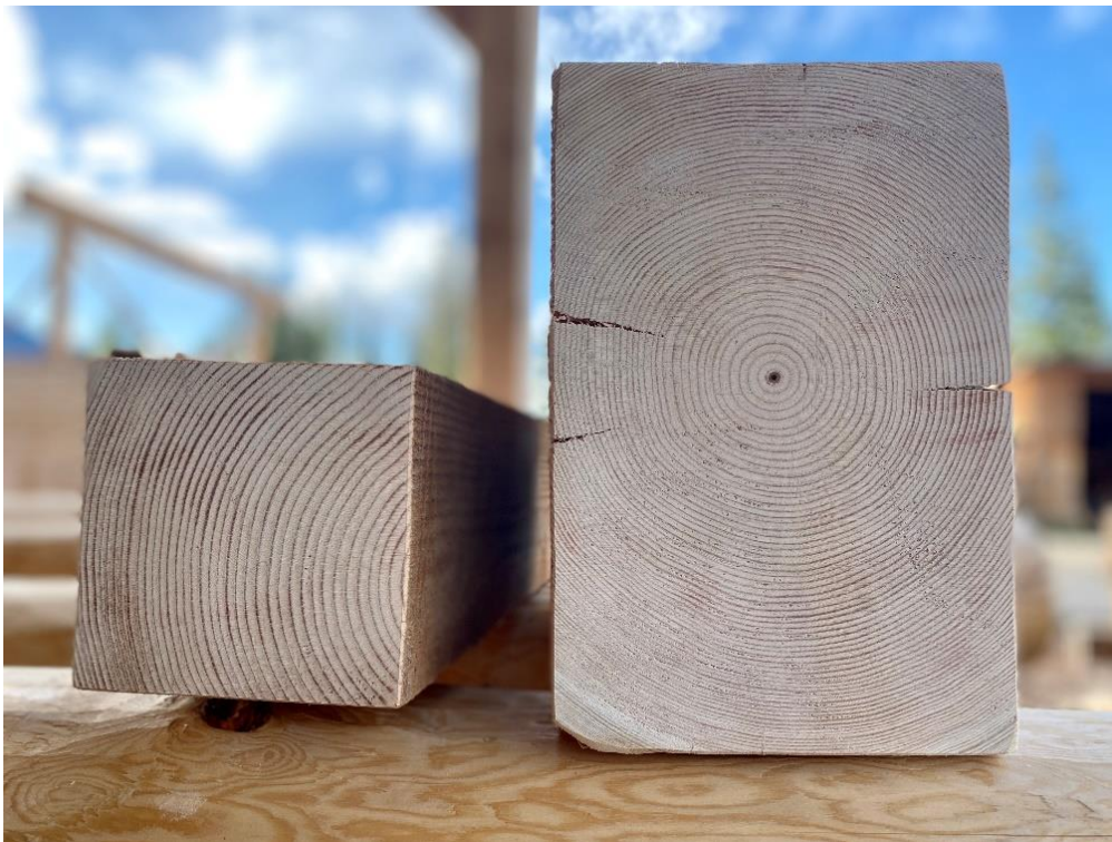
Free of heart centre (left) and boxed heart (right) timbers.
